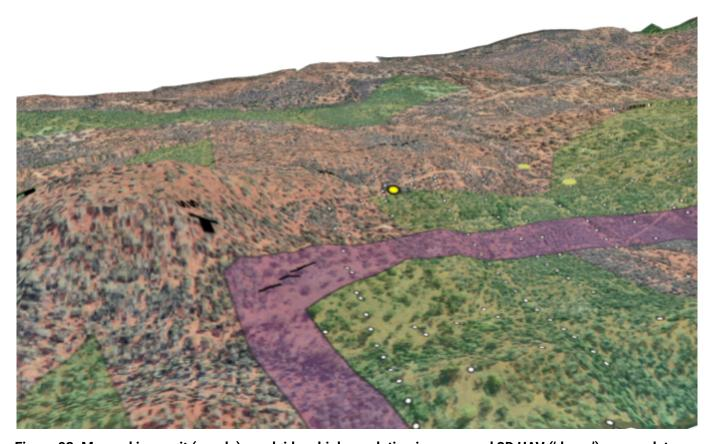
Figure 03: Mapped iron unit (purple) overlaid on high resolution imagery and 3D UAV ('drone') survey data
